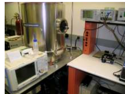
Power amplifier in TVAC chamber (LGS)
