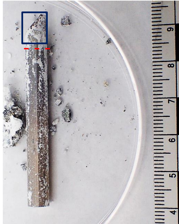
WE43 rod analyzed with CT. Red dotted lines indicates areas of transverse sectioning on CT images.
