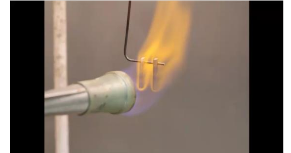
FAA testing on WE43 in air. Video provided by Luxfer MEL Technologies.
