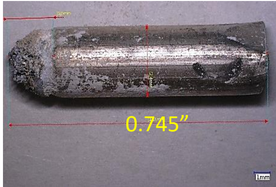
AZ31 3/16" thick rod analyzed using the digital microscope. Scale as shown.
