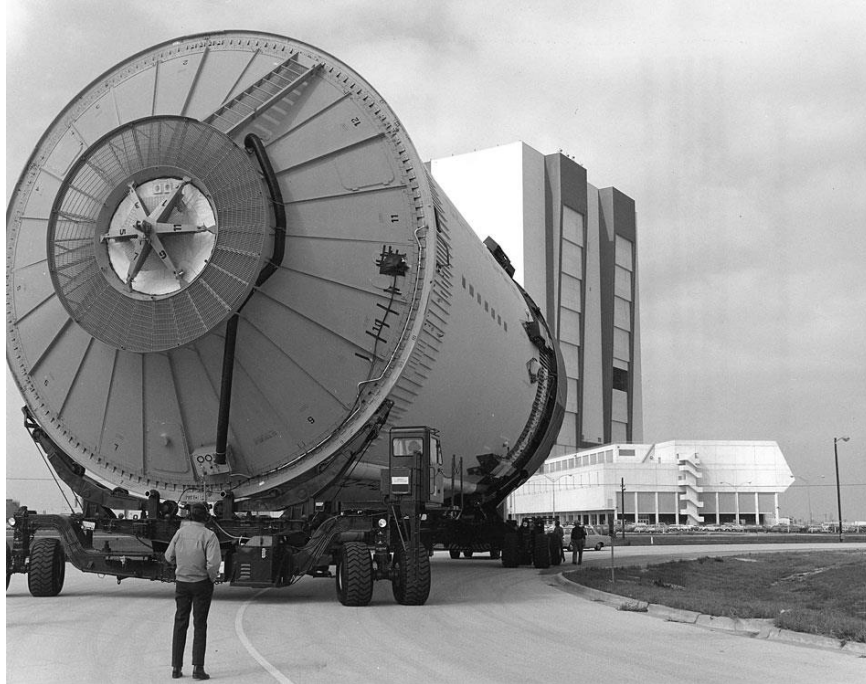
Figure 1. The Saturn V second stage moves over roads at KSC, using GSE hardware (Reference 1).
