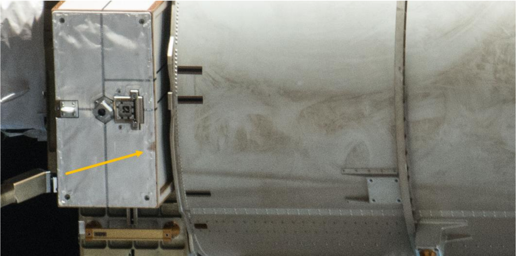
MLI Damage and Discoloration on S6 Mast Canister
