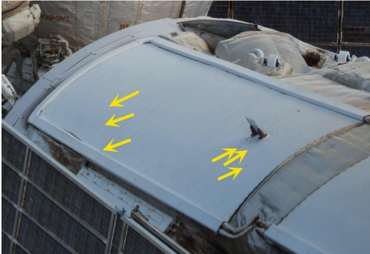
Possible MMOD Strikes or Paint Chips on FGB; Nadir
