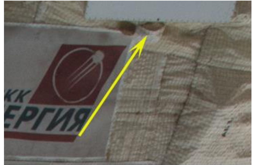
Possible Torn MLI Near Energia Label on MRM2 Forward/Port
