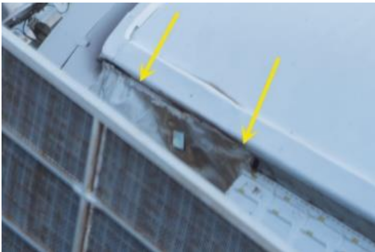
Discoloration Observed on FGB MLI Next to Radiator; Plane 1 /Nadir
