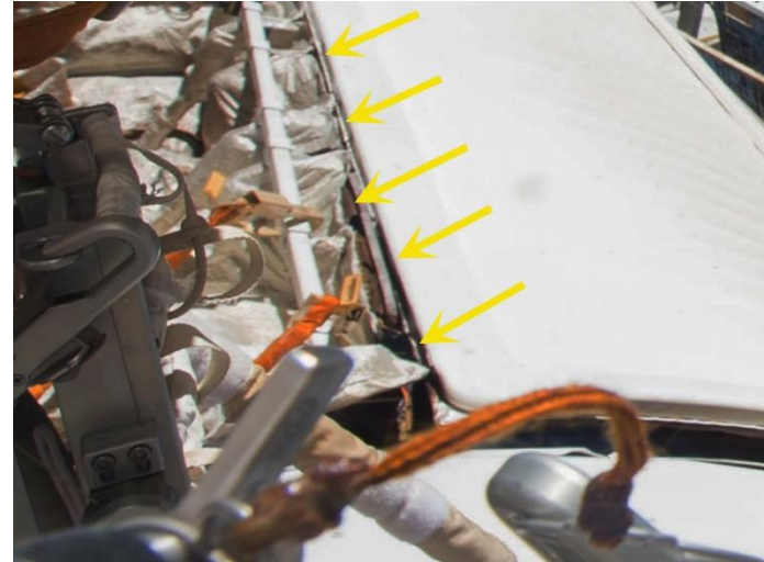
Possible MLI Lifted on FGB; Plane 3 /Zenith
