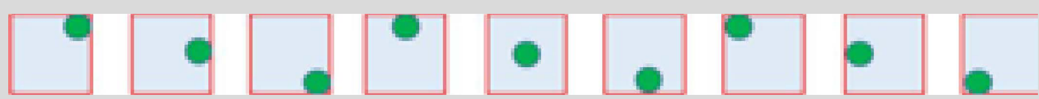
Figure 1 – Example of super-resolution algorithm using 9 input images that differ in subpixel shifts. The middle pixel being reference
