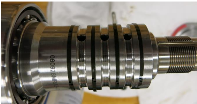
Figure 13. RFT Shaft Mounted Rotor and Ring Seals.
