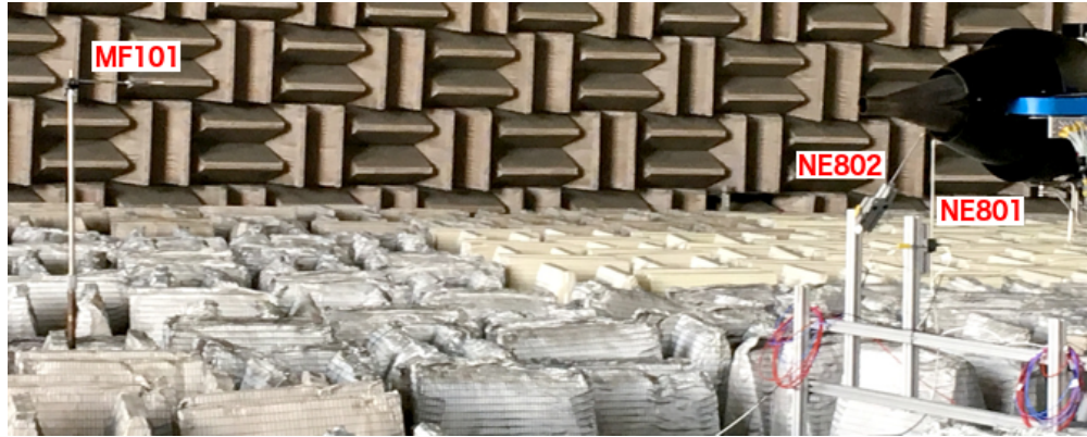
Figure 2. MF101 midfield microphone; NE801 and NE802 ITPs at DART core exit
