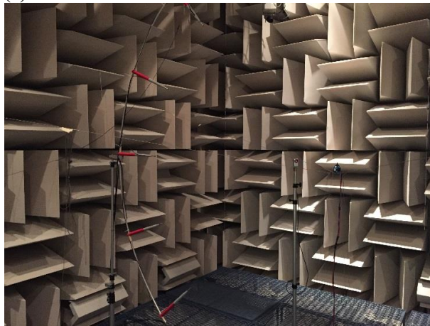
Figure 1. Acoustic Test Laboratory (ATL) at the NASA Glenn Research Center. (a) Schematic. (b) Picture of ATL with motor and microphone array.
