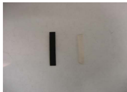
Recovered Permanent Shape, T < T_g
