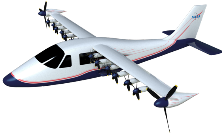
Figure 1: NASA's Scalable Convergent Electric Propulsion Technology Operations Research (SCEPTOR) final Mod IV fully electric X-57 aircraft concept with distributed propulsion.
