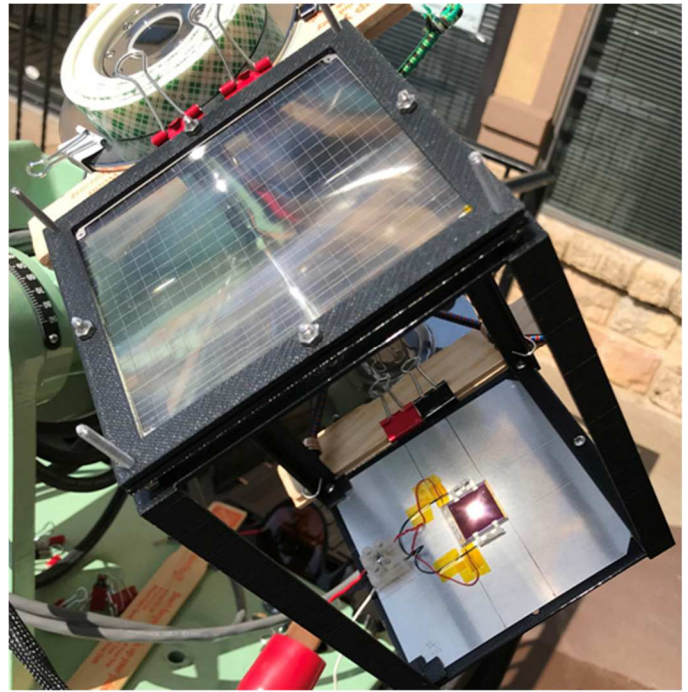
Fig. 2. Outdoor Testing of New Titanium Mesh Lens and others have used in the past for terrestrial solar concentrators. We first measure the short-circuit current of the cell with the lens in place. We next measure the short-circuit current of the cell with the lens replaced with a black plate with a square aperture hole to allow only direct sunlight to hit the solar cell, while blocking diffuse light, as shown Fig. 3. The sides of the concentrator are also covered with a black material
