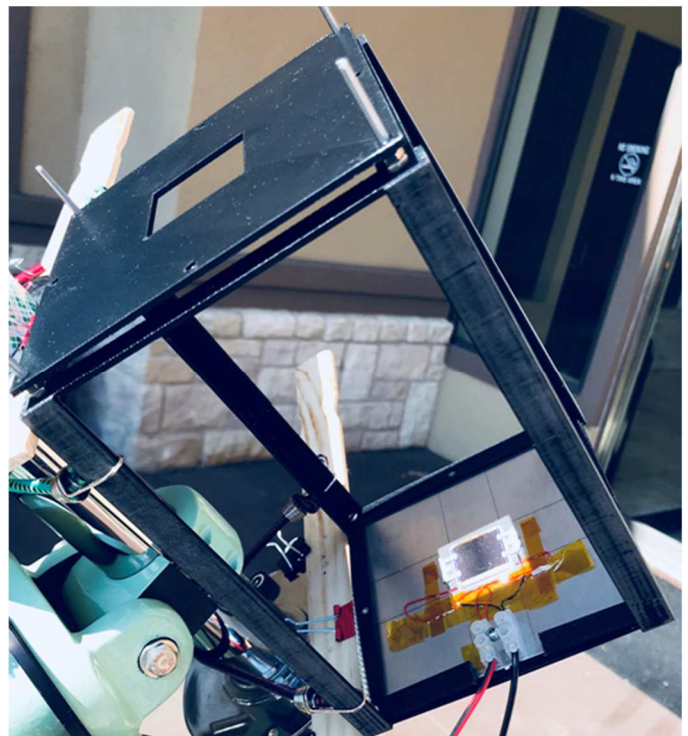
Fig. 3. One-Direct-Sun Outdoor Test.
