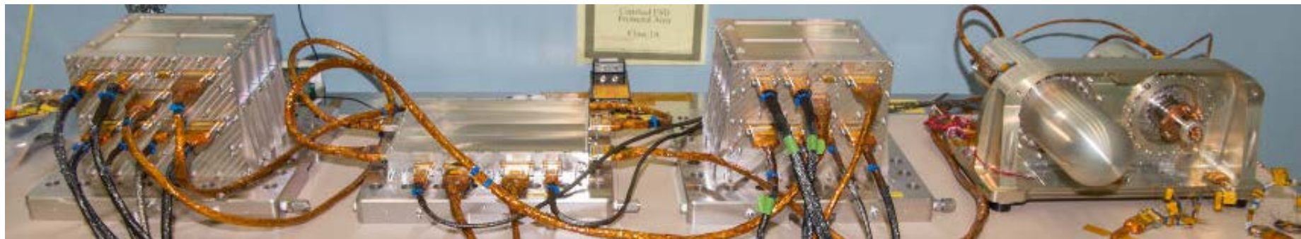
Flight Cryocooler Control Electronics, Redundancy Switch Electronics, and Thermal Mechanical Unit at GSFC
