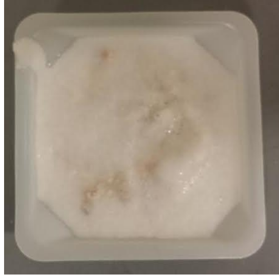
Fig. 9 As casted large (4x 4 cm) sample using low melting organic eutectic. This sample has annealed mixture
