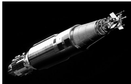
Fig. 2 SNAP-10 Reactor and Flight System Concept
