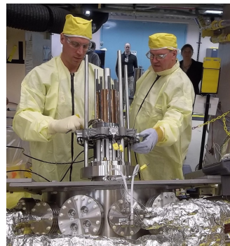
Fig. 3 Kilopower Reactor Concept and Test Unit Assembly
