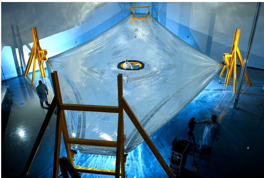
The Webb telescope project is developing a series of template sunshields with successively higher fidelity. This full-scale sunshield membrane is arranged on a test fixture to test its three dimensional shape. [Northrop Grumman Aerospace Systems]
