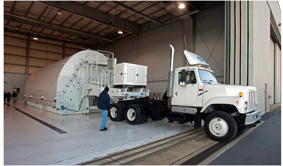
The ivory-colored semi-cylindrical aluminum trailer will be used to move components of the telescope within the US and transport the telescope to French Guyana. The trailer measures 18.5-feet wide by 17-feet tall. [NASA/Desiree Stover]
