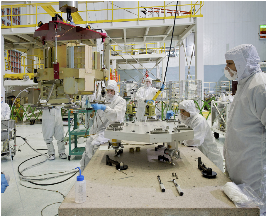
Above: Webb's Fine Guidance Sensor and Near-Infrared Imager and Slitless Spectrograph (FGS/NIRISS) was built by the Canadian Space Agency and recently delivered to NASA's Goddard Space Flight Center. In this image, the instrument is being lifted for placement on a master tool for key measurements prior to installation onto its flight structure. [NASA Goddard/Chris Gunn] Right: Webb's Near-Infrared Spectrograph, seen here undergoing testing, was contributed by the European Space Agency. [Astrium/NIRSpec]
