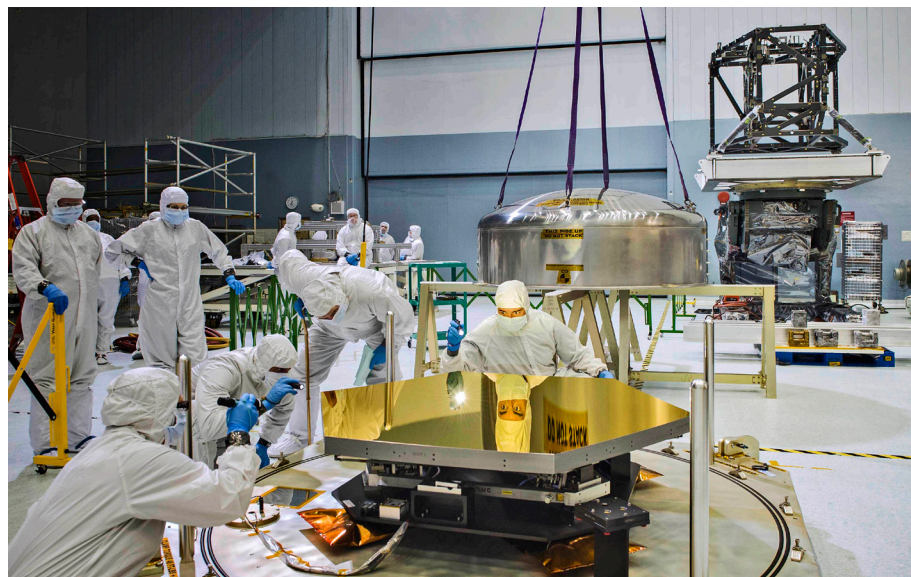
Top: A fully functional, 1/6th scale model of the Webb mirror in an optics test bed. [Ball Aerospace] Above: Webb's mirror segments are made of beryllium and coated with gold. In this photo, engineers are using flashlights to inspect a mirror segment after shipment to Goddard. [NASA/Chris Gunn]
