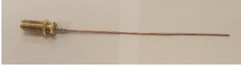
Fig. 3 The 104 mm short wire antenna
