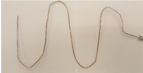
Fig. 4 The 30 cm long, curved wire antenna
