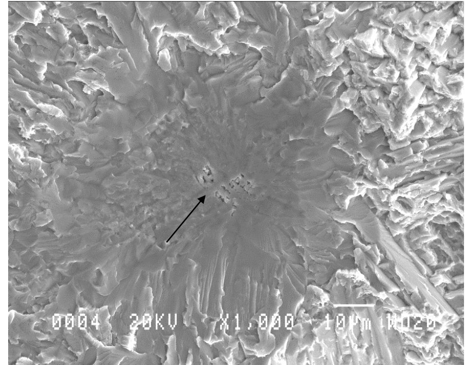
Initiation at pores probably a result of argon entrapment during powder processing
