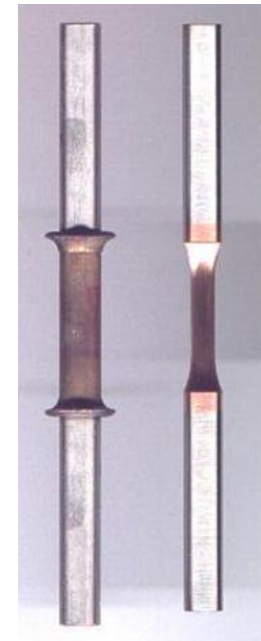
LCF samples with welded ends
