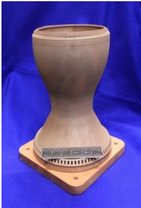
GRCop-84 Combustion chamber
