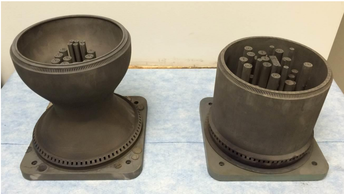
Chamber builds with coupon samples
