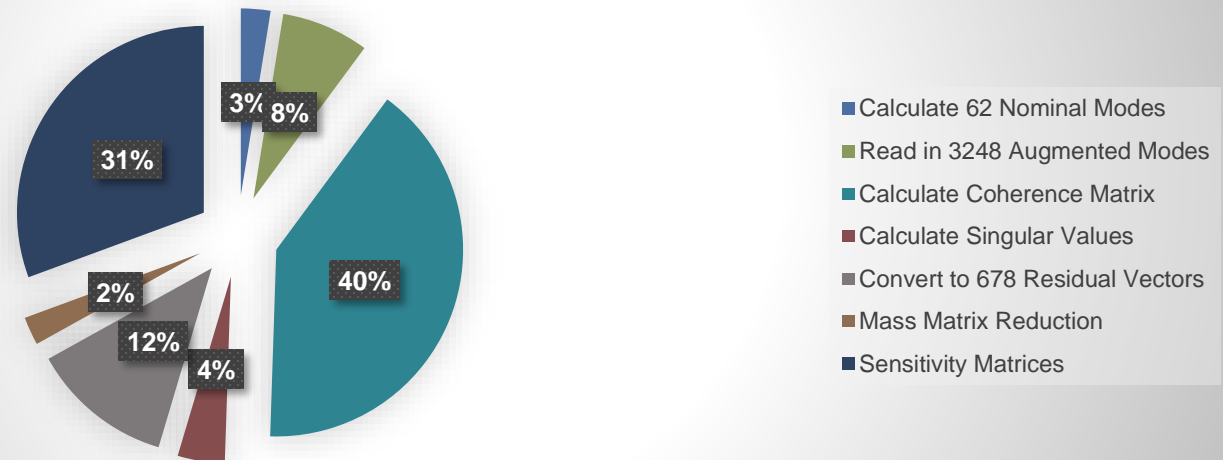
Nastran RunTime Breakdown Out of 859 Seconds for 62 Normal Modes and 678 Residual Vectors
