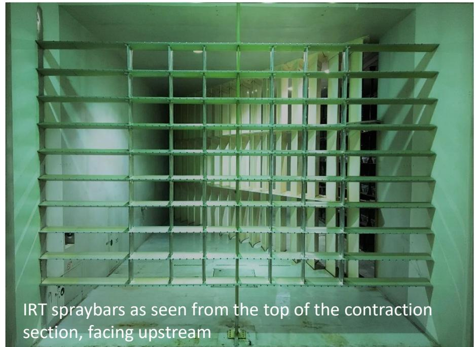
IRT spraybars as seen from the top of the contraction section, facing upstream
