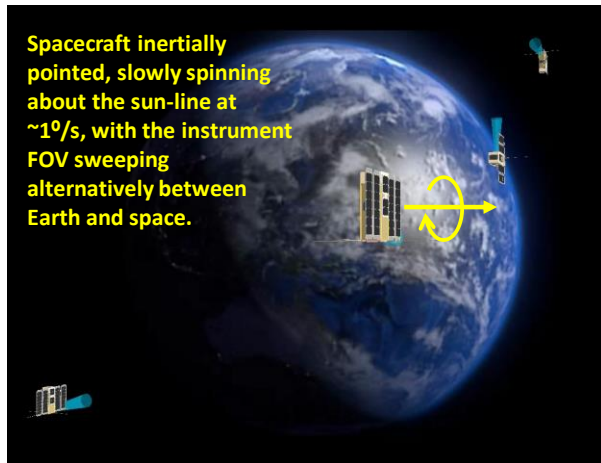
Figure 4: Typical operations over one orbit, with alternate Earth/space views for calibration
