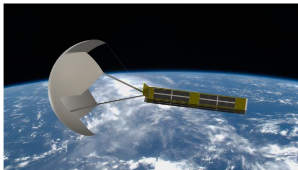
Figure 13 TechEdSat-8 is a linear-6U Flight Demonstration Platform (Modulated Exo-Brake Drag Device) for Advancing Telemetry Experiments
