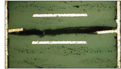
Delamination between copper conductors, core and prepreg 1
