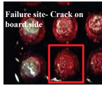
(a) Failure on board side
