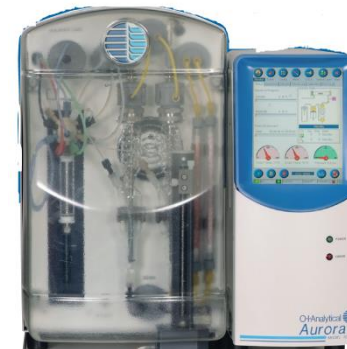
OI /Xylem Aurora UV Combustion or UV Persulfate / NDIR
