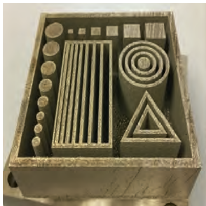
FIGURE 1. CAD model and SLM IN-718 build showing subsurface defects.
