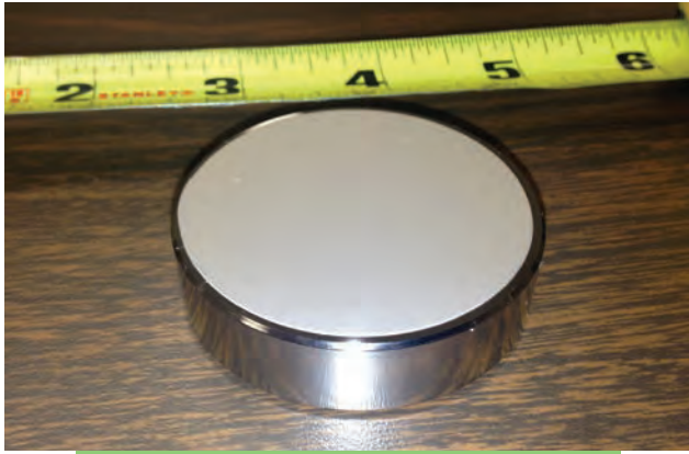
FIGURE 2. The first hybrid ceramic optic was produced on a 2-in-diameter flat. The low-frequency figure of the sample appeared to be negatively influenced by the shrinkage mismatch between the ceramic and electroformed NiCo, however.
