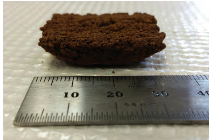
FIGURE 2. First sodium silicate Mars brick. Photo provided by Dr. Richard Grugel.
