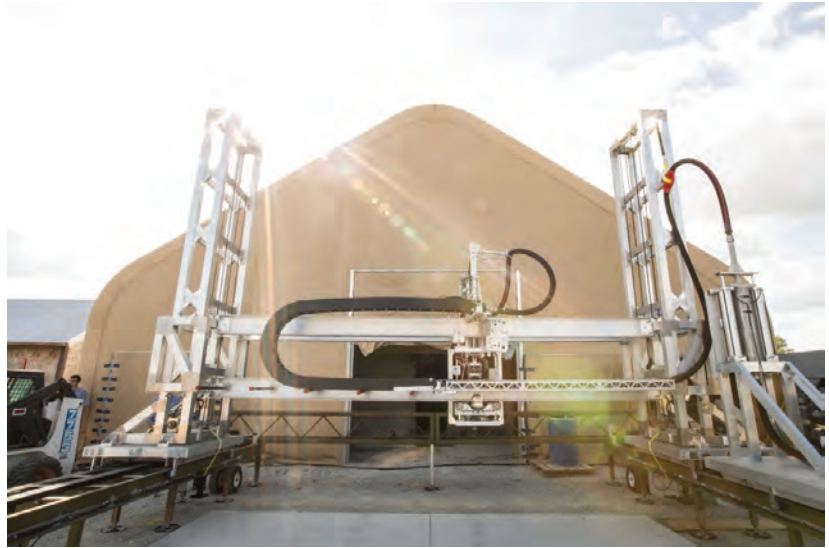
FIGURE 2. The ACES-3 gantry system designed and built by MSFC provides mobility.
