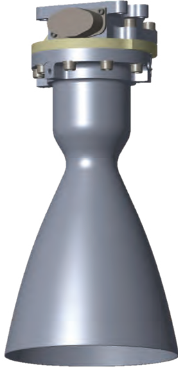
FIGURE 2. Deep Space Engine CAD rendering.
