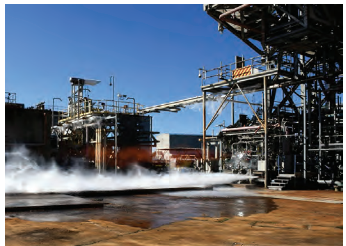
FIGURE 2. A hot-fire test of Unit 3 occurred on November 9, 2017. The chamber pressure reached 900 psi and produced 17,000 lbf of thrust.
