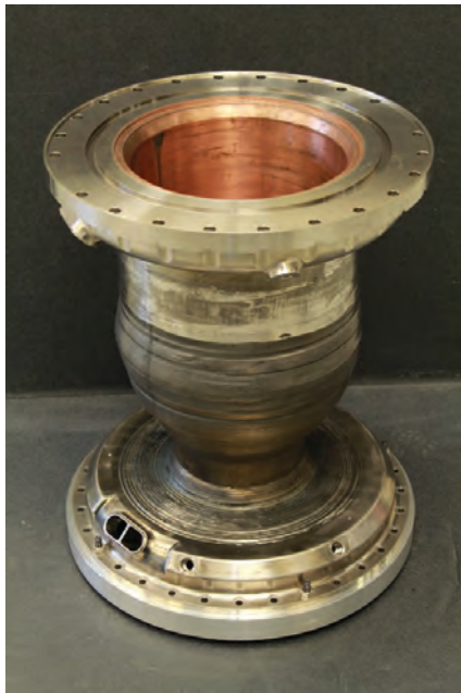
FIGURE 1. Combustion chamber showing the bimetallic bond of GRCop-84 liner and the Inconel 625 structure jacket and manifolds.
