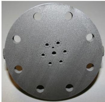
100lb LOX/Propane Nanolaunch Injector. Built 2012. Tested 2013.
