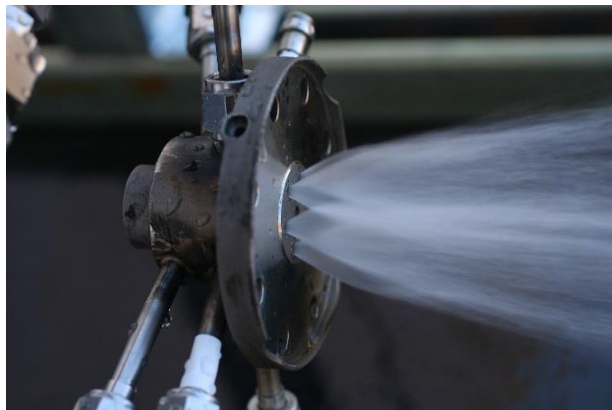
Nanolaunch Injector Water Flow Test
