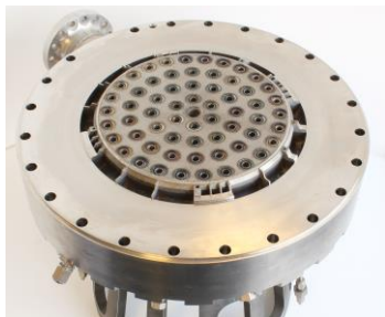
35K AMDE Injector with Welded Manifolds, Tested 2015
