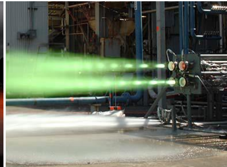
Four Thrusters with 1200 lbf Shear Coaxial Injectors.
