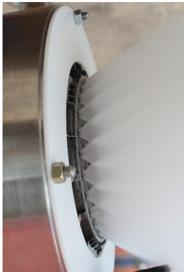
Water Flow of the AMDE Injector LOX Circuit; Hot Fire Test of the AMDE Injector.
