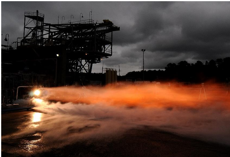
Water Flow of the AMDE Injector LOX Circuit; Hot Fire Test of the AMDE Injector.
