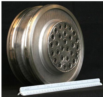
20K LPS Subscale Injector. Tested August 2013
