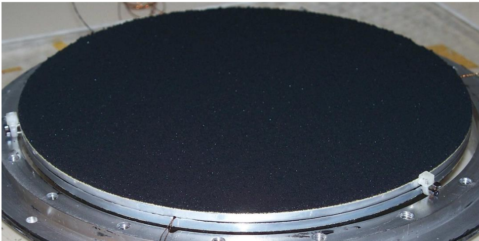
Two sample halves epoxied together
