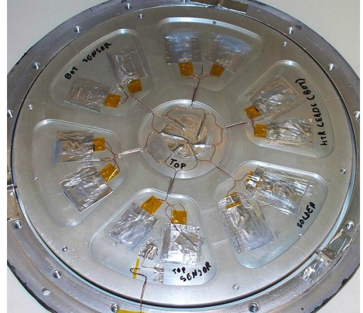
Sample heater elements epoxied/taped
