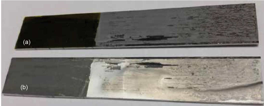
Figure 14.—Specimen 3-2. (a) Top half polymer matrix composite. (b) Bottom half shape memory alloy.
