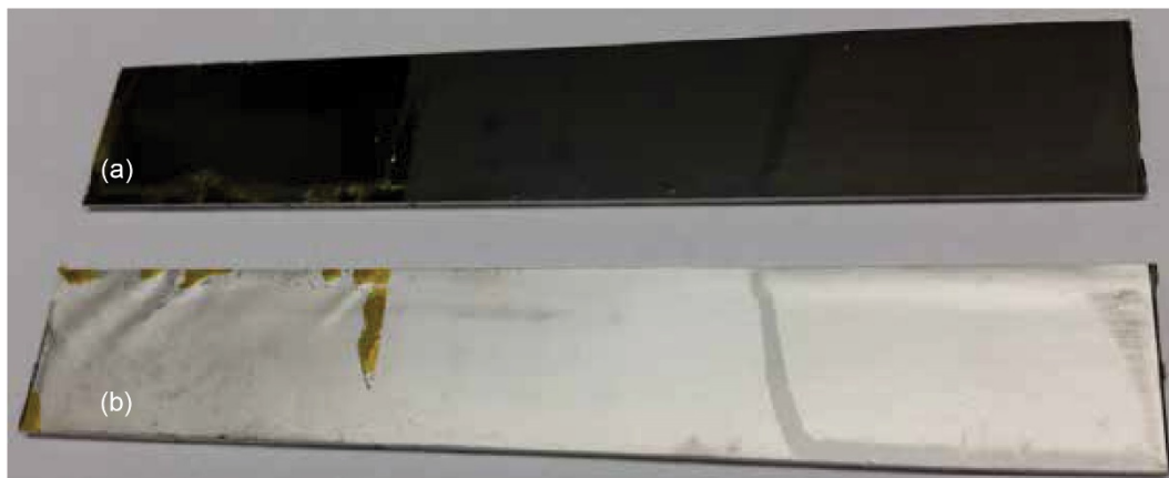
Figure 13.—Specimen 2-1. (a) Top half polymer matrix composite. (b) Bottom half shape memory alloy.
