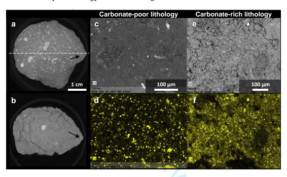
Figure 2. Optical photos of the Tagish Lake meteorite sample before and after the heating experiment at 900°C for 96h. The sample shows significant weight loss (~20%) upon heating which indicates the dehydration of phyllosilicates. Common mineral phases observed in the matrix of the unheated carbonate-poor lithology of the Tagish Lake meteorite such as phyllosilicates, magnetite and Fe-Ni sulfides were converted into anhydrous silicates, Fe-Ni metal and troilite via dehydration and reduction.
