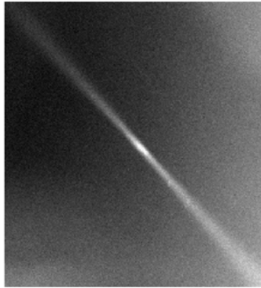
Figure 2. Sample raw Rayleigh scattering image. Conditions are P = 445 kPa, T = 271 K, and M = 0.4 .
