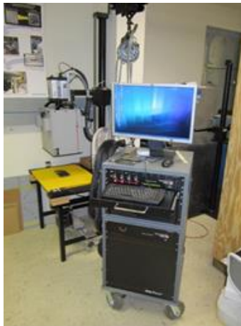
Figure 1. Photograph of the flash thermograph system.
