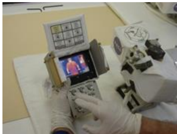
Figure 4. Infrared inspection system designed for on-orbit inspections.
