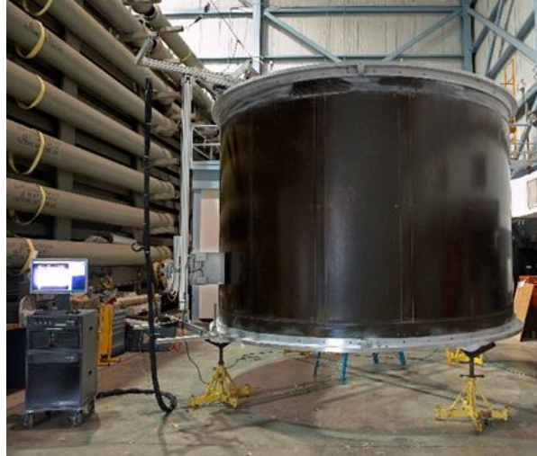
Figure 2. System configured for large area inspection of a composite test article.
