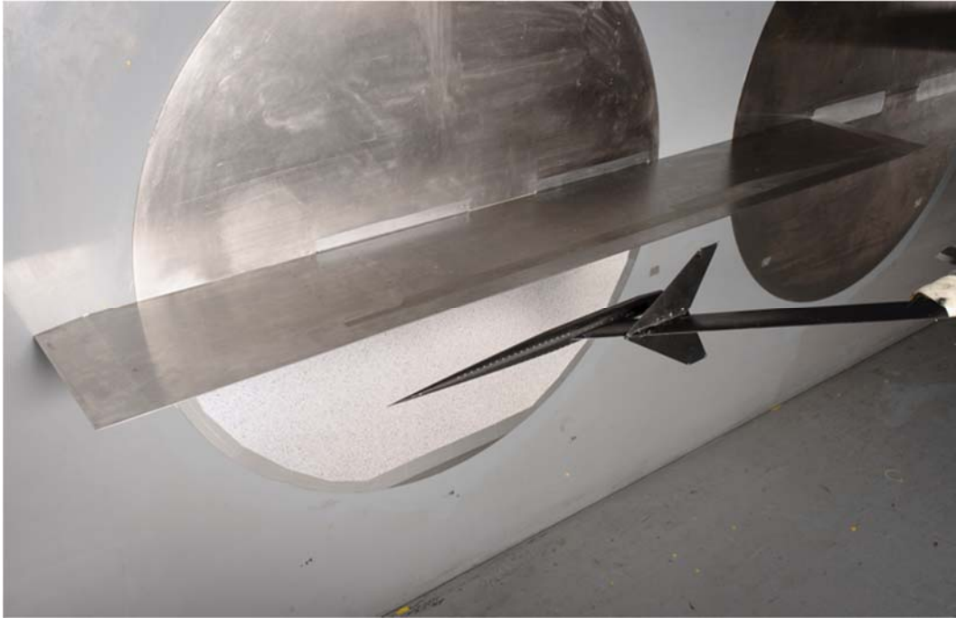
Figure 2. Photograph of the plume/shock interaction model above the 14" pressure rail, with the 25-D tail installed on the blade strut.
