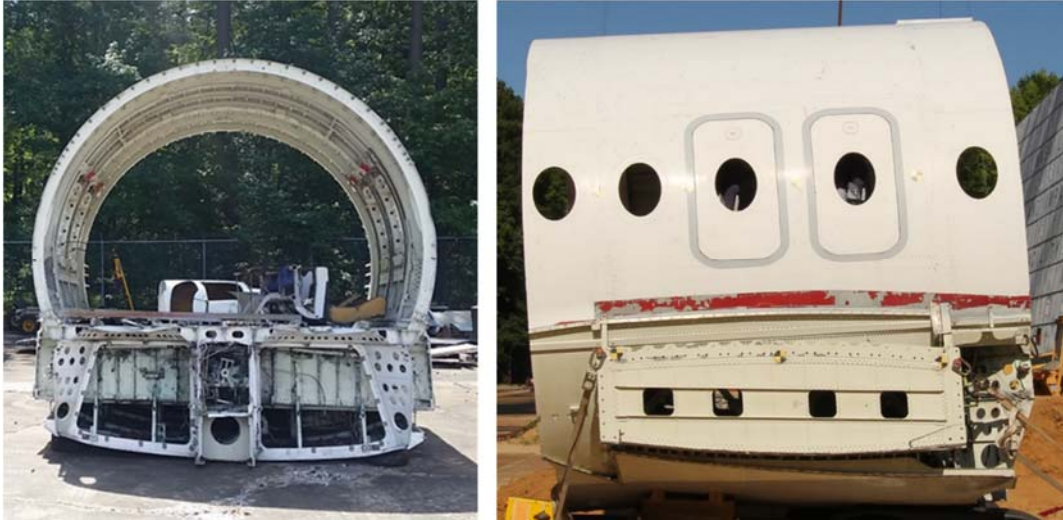
Figure 2 – Un-Instrumented F28 Wingbox Section aft view (left), and port side view (right)
