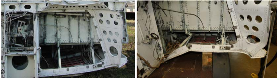
Figure 6 - Lower aft cavity. Before test (left) and damage post-test (right)
