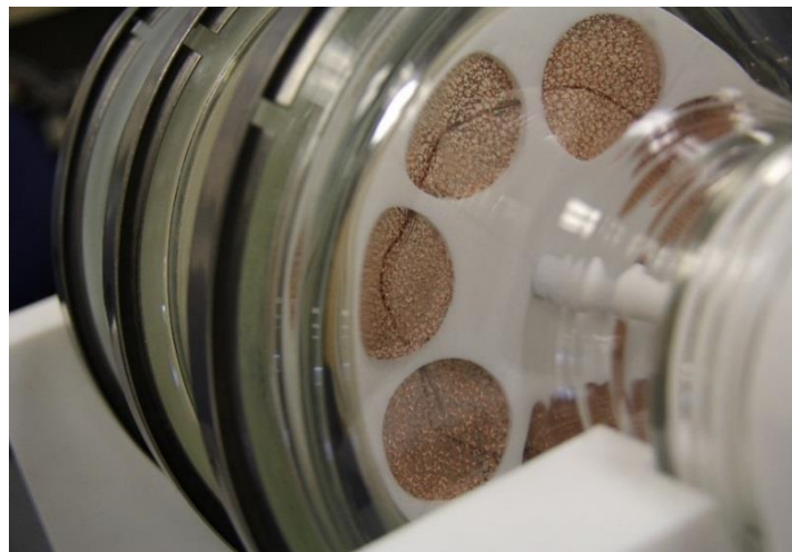
Figure 3. Cathode chamber containing Cu substrates with electrical connections.
