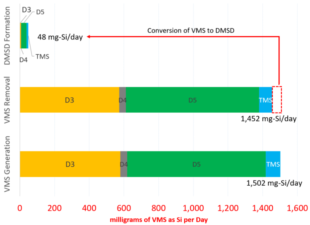
Figure 4. Generation, Removal, and Reaction of VMS Compounds to DMSD. 13
