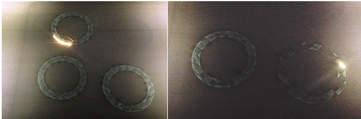
Figure 4. SLM Chamber Fabrication showing the Coutouring Pass (Left) and In-fill Pass (Right).
