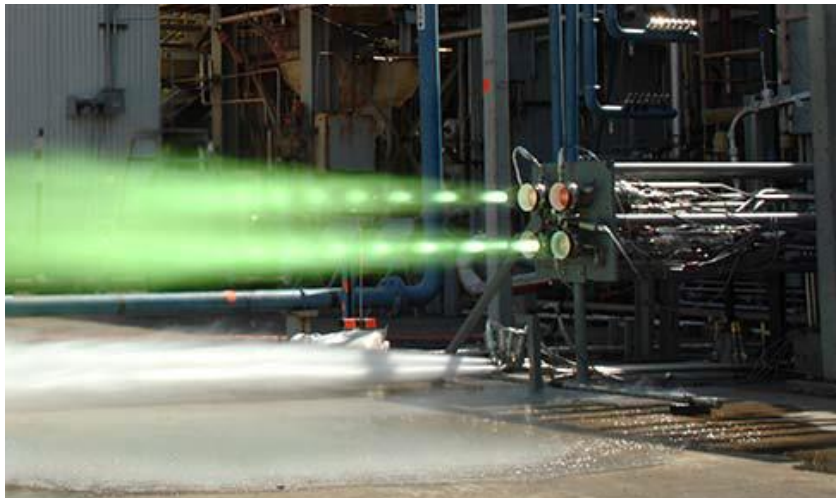
Figure 10. Cluster of Four Thrusters with 1200 lbf Shear Coaxial Injectors.
