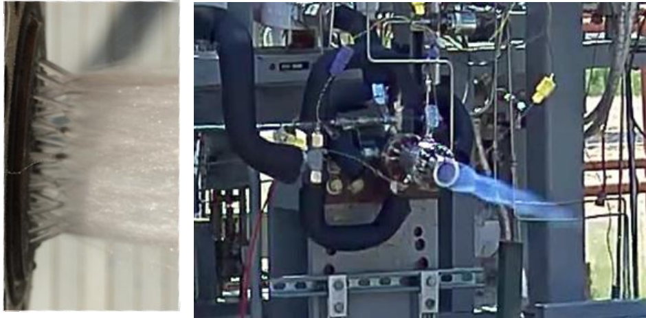
Figure 11. Water-flow of FOF element injector for a LOX/CH 4 Gas Generator (left); Hot-fire test (right).
