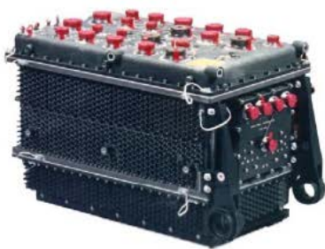
SSME Engine Controller
