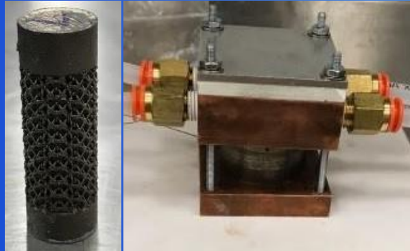
Thermal conductivity specimen and experimental test apparatus based on modified ASTM 1225-04.
