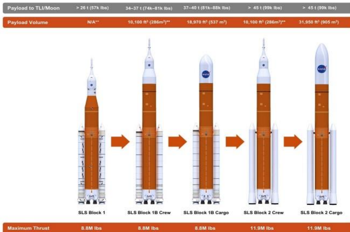
Figure 14. The Block 1 configuration is the first variant of the SLS family of vehicles that will provide the performance and payload capacity to lift Mars-class payloads.
