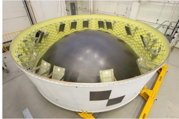
Figure 8. The finished OSA for EM-1 before it was shipped to EGS; mounting brackets for smallsat COTS dispensers and an avionics box are visible just above the diaphragm.
