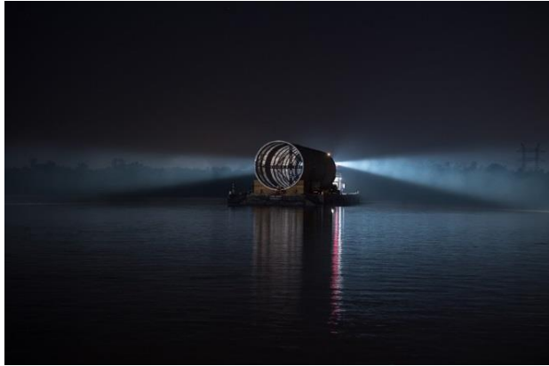
Figure 10. The SLS Program elected to build a “pathfinder” of the same dimensions as the core stage to give ground support and transportation crews experience in transporting and handling full-size spaceflight hardware.
