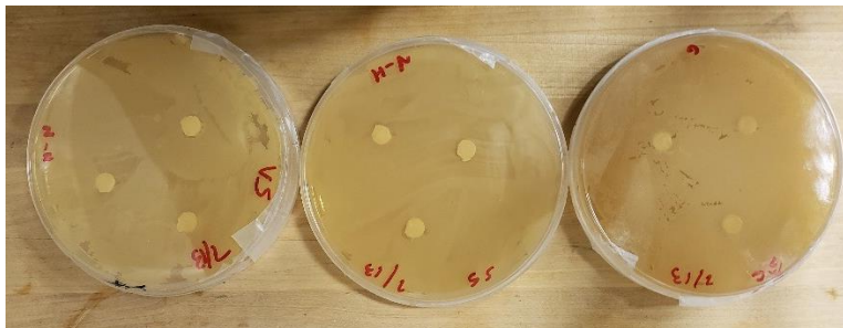
Figure 6: Kirby Bauer tests done on Royco® 43 SAE AMS-G-4343 with three different species of bacilli showing no zones of inhibition.
