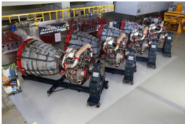
Fig. 6 All four EM-1 RS-25 engines have been tested and verified; they are ready for integration into the core stage and flight.
