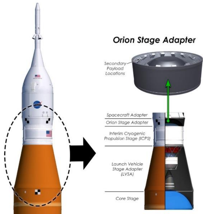
Fig. 2 At the top of the Block 1 configuration, the Orion Stage Adapter (OSA) has capacity for 13-17 smallsats.
