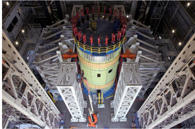
Fig. 5 Engineers installed structural test hardware for the SLS core stage intertank into a stand at Marshall Space Flight Center, where testing recently began.
