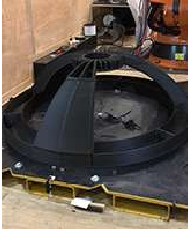
Figure 5. Dome 3D-printed by Foster+Partners/Branch Technology at the phase II, level 3 head to head competition.
