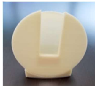
REM Shield Enclosure: Enclosure for radiation monitors inside Bigelow Expandable Activity Module (BEAM). Printed 3/20/17 (1 of 3). Others printed 5-30 and 6-16. All are now installed on BEAM.
