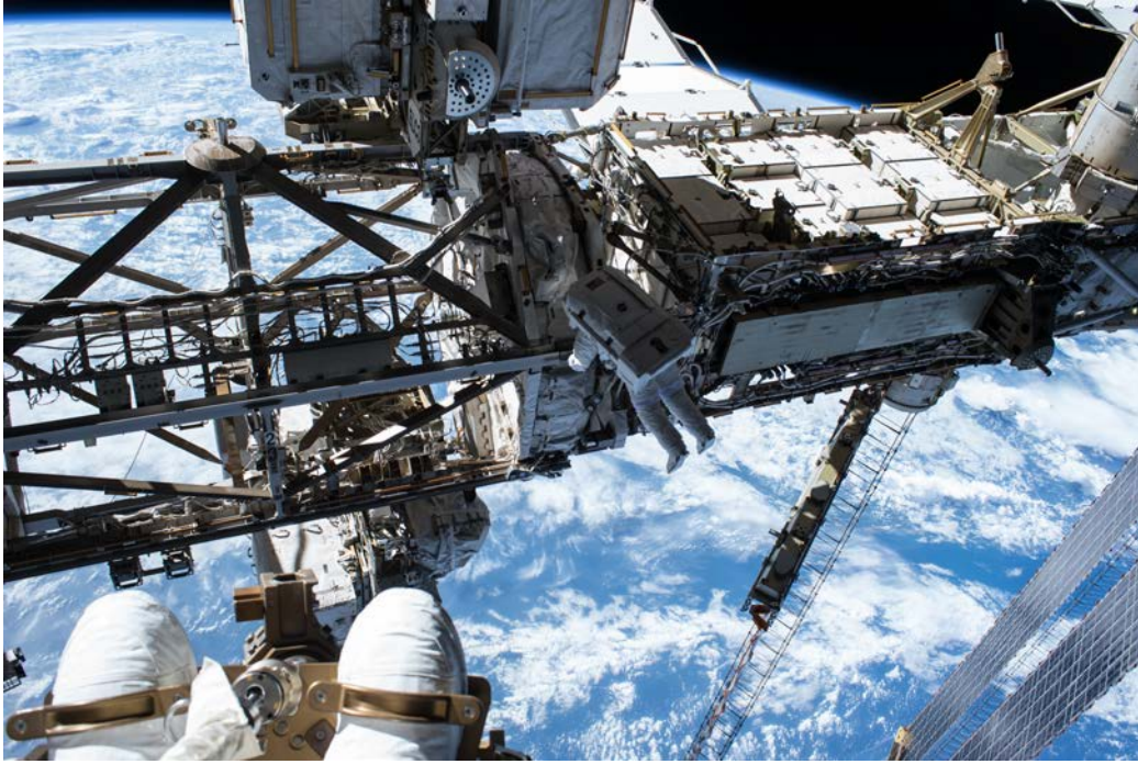
Figure 1. An ISS truss with exposed C&DH and power cables as imaged during an Expedition 48 extravehicular activity (EVA) of Commander Jeff Williams and Flight Engineer Kate Rubins [7].
