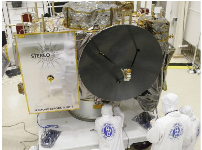
Figure 4. STEREO High Gain Antenna 1.2m parabolic dish
