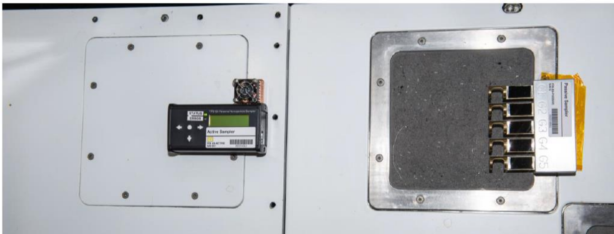
Fig. 8 Active (left) and Passive (right) samplers deployed in Node 3 aboard ISS [32]
