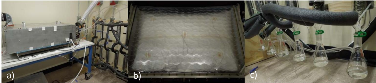
Fig. 4: Prototype BPA testing at Paragon in Tucson. a) Prototype assembly; b) Brine-filled bladder installed in the detrusor; c) Condensate collection during a prototype dewatering test [24]
