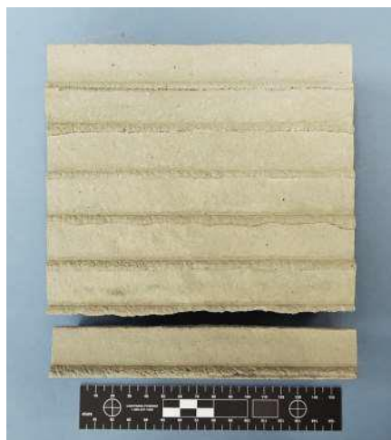
Figure 1. Additively constructed sample in which layer adhesion between a dry mortar layer and a wet mortar layer added the following day was proven to be weak compared to layer adhesion between two wet mortar layers emplaced on the same day.
