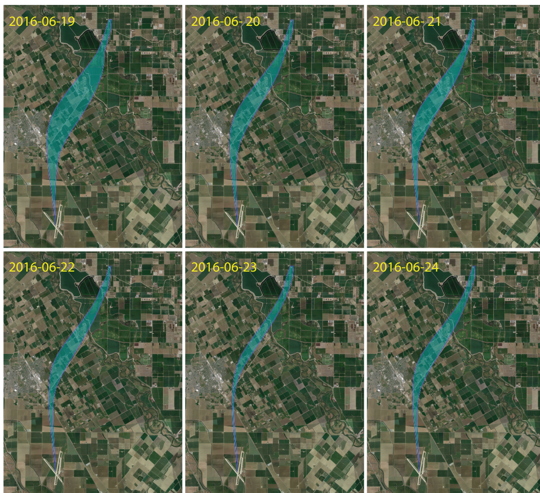
Figure 3. Simulation using wind data from 2016-06-19T00:00:00Z to 2016-06-24T23:59:59Z at NASA Crows Landing, CA. For each day we compute the mean trajectory and two bounding trajectories (shown in dark blue) based on the standard deviation.
