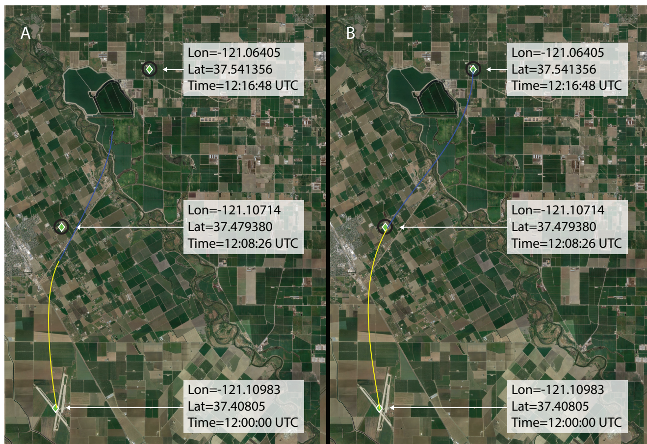
Figure 2. Client provides waypoint information including the arrival times at each waypoint. The trajectory estimator then generates an expected trajectory given waypoints and vehicle data at cruise velocity. In addition, optimization is performed over the range of velocities specified in Table 1 in order to determine feasibility of the submitted flight plan.
