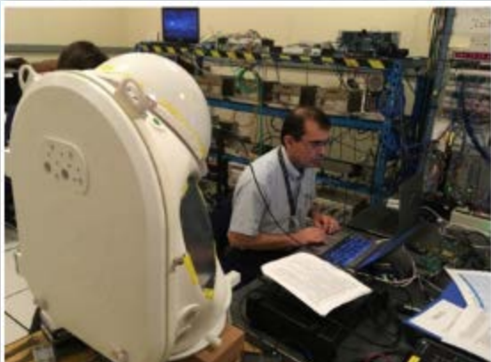
Integrated Communications Testing Z-2.5 3D Printed HUT
