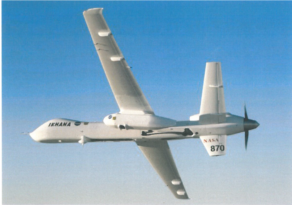
Figure 1a. Ikhana unmanned aircraft (66-ft wingspan) (ref. 10).
