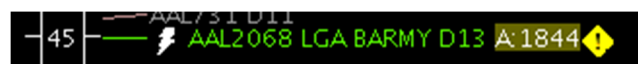
Fig. 11. STBO Client timeline display of approved APREQ release time different from originally requested time.
