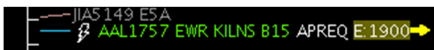
Fig. 8. Yellow arrow on STBO Client timeline indicating APREQ release time request has been sent.
