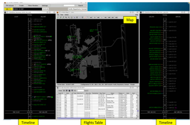
Fig. 2. STBO Client interface, showing the toolbar, map, flights table, and timeline features.
